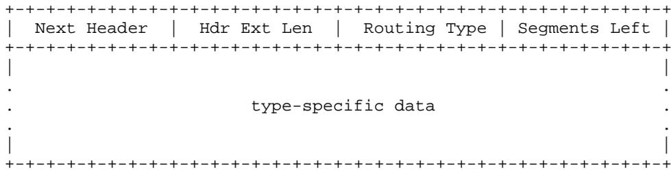
Next Header: It is 8-bit selector. It identifies the type of header immediately following the Routing header.
