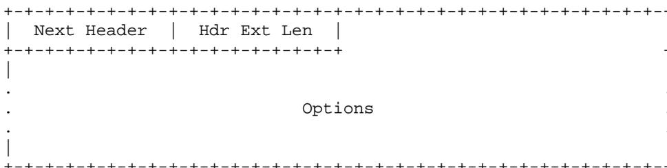
Next Header: It is 8-bit selector. It identifies the type of header immediately following the Destination Options header.
