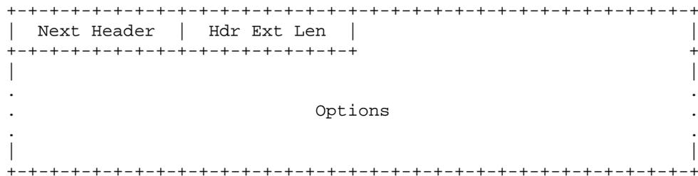
Next Header is of 8-bit size. It identifies the type of header immediately following the Hop-by-Hop Options header.
