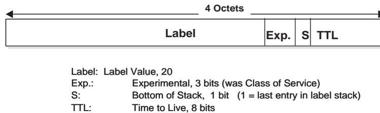
**Figure 1.3** MPLS “shim” header format
