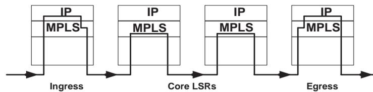
**Figure 1.5** MPLS Forwarding: Ingress LSR extracts layer 3 information, assigns packet to FEC, pushes a label and forwards the packet. Core LSRs use label forwarding. Egress LSR pops the label, extracts layer 3 information and forwards the packet accordingly
