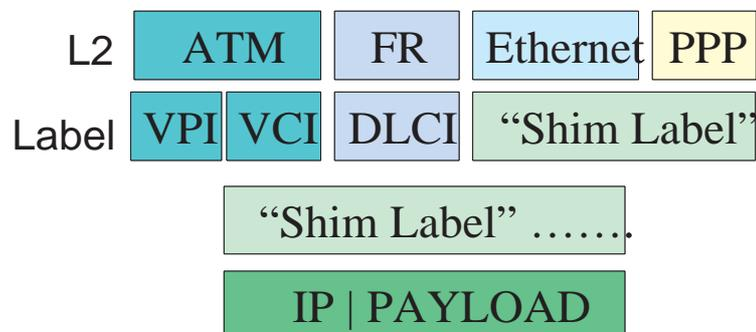
**Figure 1.6** Label encapsulation
