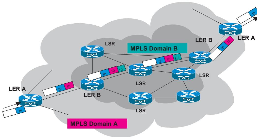
**Figure 1.7** Label Stack. LERs A are for MPLS domain A and LERs B are for MPLS domain B
